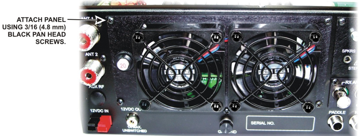
Figure 17. Fan Panel Installed on K3.
