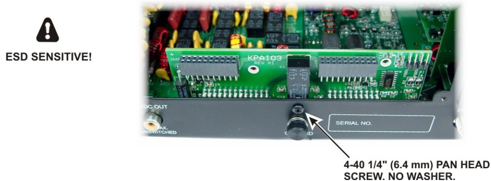
Figure 11. Installing the KPAIO3 Module.
