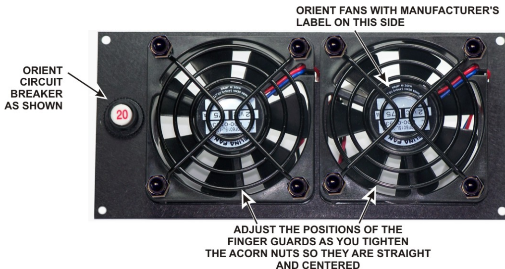
Figure 13, Completed Fan Panel from Rear.
