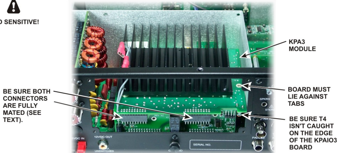
Figure 15. Mounting the KPA3 Module.
